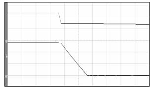
Figure 6 Output voltage shut down by power off, (5ms/div), see Figure 10 for test configuration; CH1-input voltage (20V/div); CH2-output voltage (10V/div)
